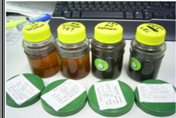
Before (right containers) and After (left containers) photo showing the result of the filtration of the synthetic oil of the wheel motor for the 787 Leibherr truck
